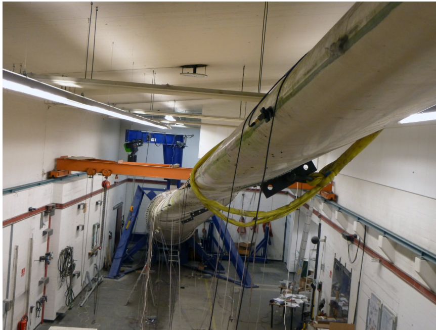
Figure 1. The real-scale turbine blade tested.
